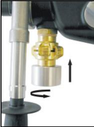
Dust which occurs during your work is hazardous to health. That is why it is advisable to use a deduster and to wear a dust mask on dry drilling. Place the adapter for the dedusting unit onto the tool's connector and turn into the direction of the arrow up to the stop. As a suitable wet/dry deduster, our DSS 25 A is available as add-on. The use of a dedusting system is also a prerequisite for optimal cutting performance of the bit (air cooling).
