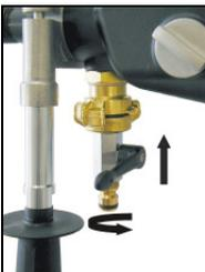
Place the adapter with the ball valve onto the tool's connector and turn into the direction of the arrow up to the stop. Connect the tool to the water supply system or a water pressure vessel using the push fit nipple. **Attention! The maximum water pressure should not exceed 6 bars. In case of higher water pressure, a pressure relieve valve must be used.**
