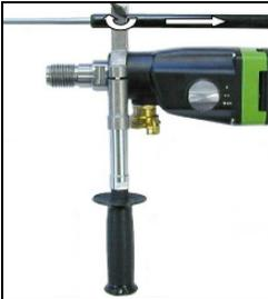
Insert the gas spring with the water collecting ring and the guide ring appropriate for the drill bit diameter into the tension disk. Shift the gas spring up to complete coverage of the bit segments by the water collecting ring. Tighten the wing screw. On drilling overhead, make sure that the water supply is opened only after having switched the water remover on and the removing unit was fixed to the wall or ceiling.
