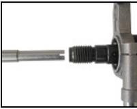
Insert the centering point so that the recesses in the centering point latch on the catches of the working spindle.
