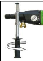
For manual drilling, the **ETN 130/3 P** may be used only together with its additional handle which comes with the tools. Place it on the gearing collar from the front and fix it by turning the handle in direction of the arrow.
